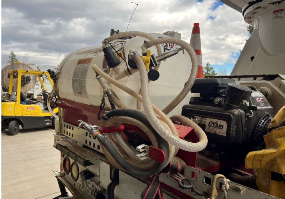
Water tanks on digger derricks for dust control and spot fire control.
